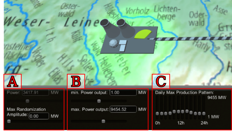
Fig. 4. The information bar for a generator node shows its current power output and the maximum output randomization amplitude (A), the minimum and maximum power output (B), and the daily maximum production pattern (C).
